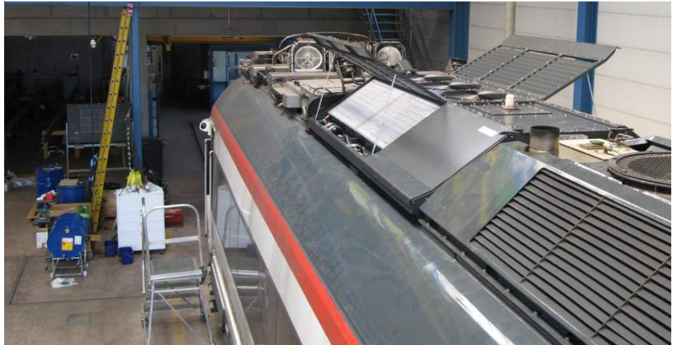
Maintenance access on vehicle
