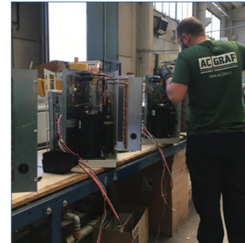
Construction of refrigeration units
