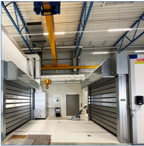
Insulated roller gates for movement from the acclimatisation chamber to the test room
