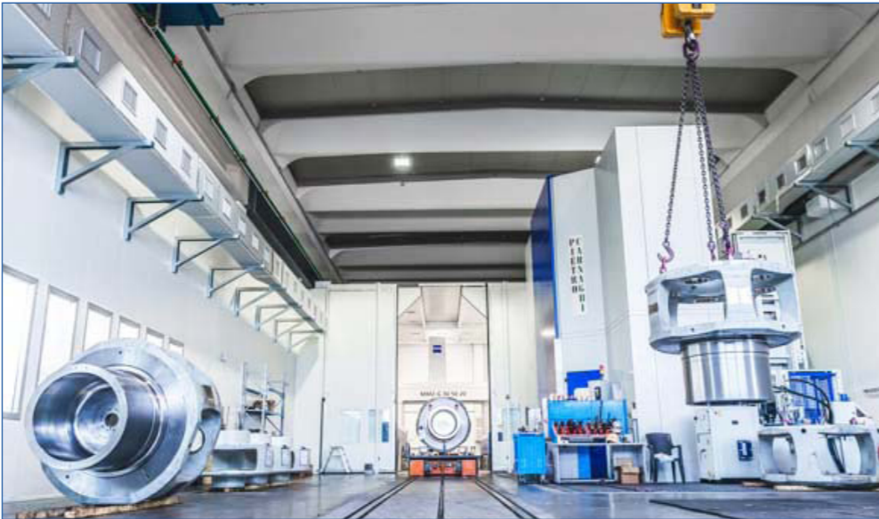
Metrology room with opening roof and rail movement carriage
