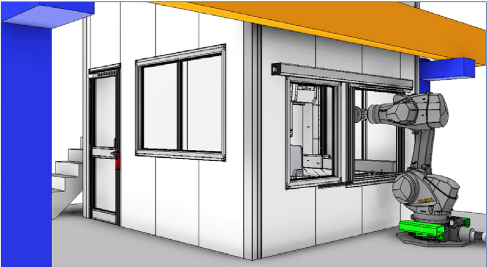
Measurement cell, automatic opening for loading/unloading robot
