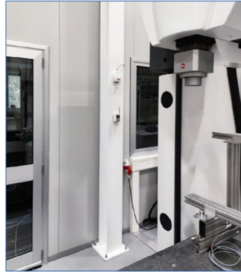
Air-conditioned chamber for the highest precision dimensional control instrument
